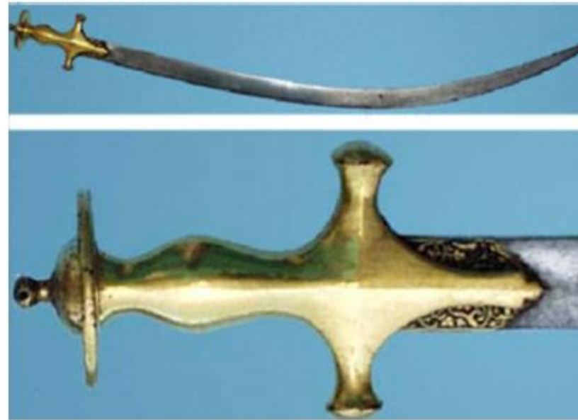
A typical sword made of wootz steel (about 18 th century); the hilt is of iron and coated with a thick layer of gold. (Courtesy: R. Balasubramaniam)
